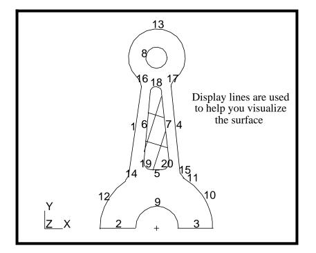
3. Chain together the outer curves in the model to create a continuous loop.
