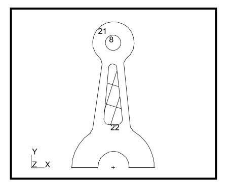
5. Create a trimmed surface using the chained curves you have created and the circular "hole" at the top of the connecting rod.
