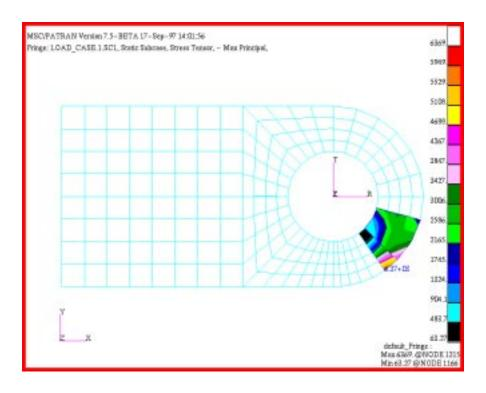
Transform Result Coordinate Frame 6. Convert the stress tensor results to the scalar  $\sigma_{xx}$ , and create a fringe plot of the scalar with respect to the cylindrical coordinate system you created when building the clevis model. Plot the results on all elements.
