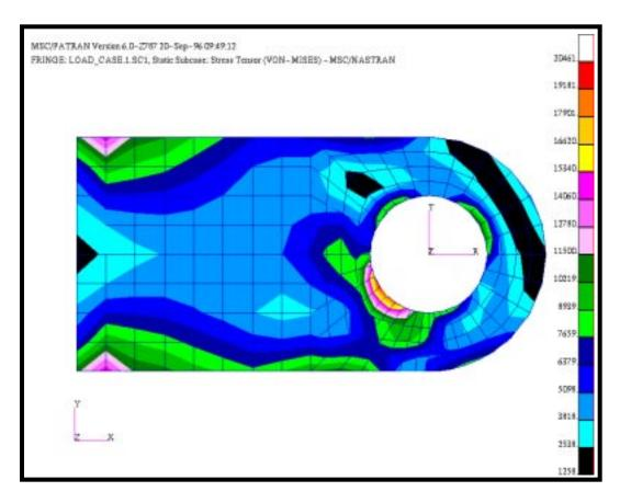
Now, let's see if the results are different using the Fringe form to plot the Von Mises stress.
