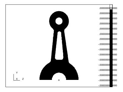
What you have just done is plot the tension in the x-direction of the global coordinate system. Write down the range of stresses in the following table. The purpose of this will become evident soon.\*
