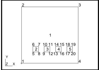
Leaving the *Action* as **Transform** change the *Object* and *Method* to **Point/Translate**. Edit the *Translation Vector* to read <0 0.0094 0> and the *Repeat Count* to 1. Click in the *Point List* box and select **Point 5** from the viewport, the lower left corner point of Surface 2. Point 21 should appear to guide layout of the remaining four devices.
