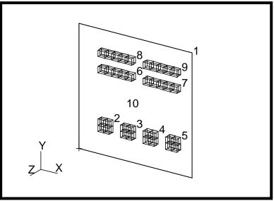
6. Mesh the remaining trimmed surface with Paver.
