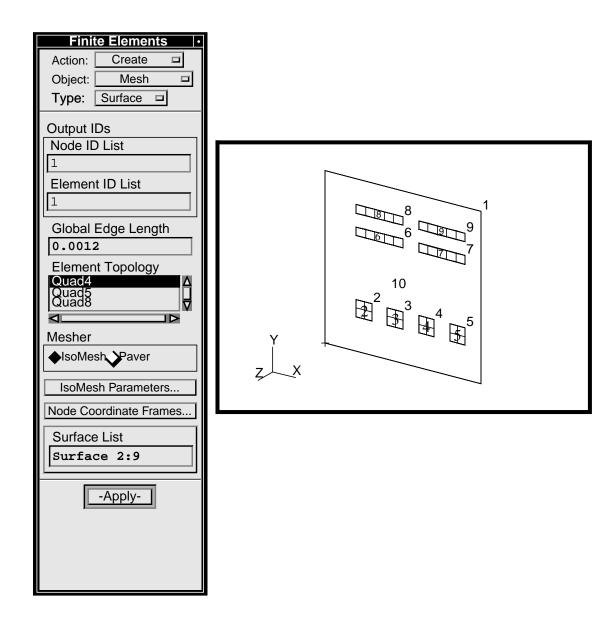
Select **Apply** to complete the meshing function. The display should appear as shown above. If it does not, select the *undo* icon and analyze the error to a resolution.
