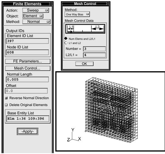
Select **Apply** to complete the meshing function. The resultant display is shown above.
