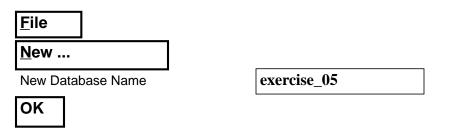
MSC/PATRAN will open a Viewport and change various *Control Panel* selections from a ghosted appearance to a bold format. When the <u>New Model</u> <u>Preferences</u> form appears on your screen, set the *Tolerance* to **Default**, and the *Analysis Code* to **MSC/THERMAL**. Select **OK** to close the <u>New Model</u> <u>Preferences</u> form.
