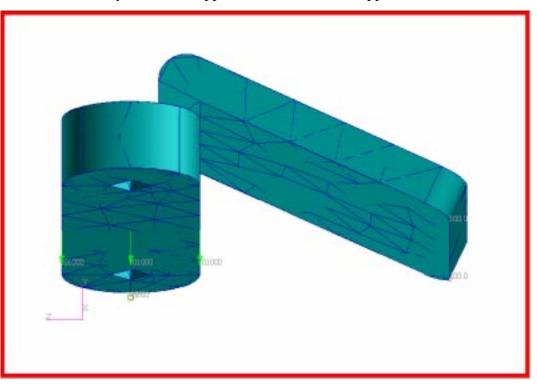
With boundary conditions applied the model should appear as shown below.
