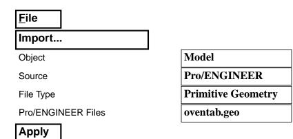
The model geometry will be imported. A <u>Pro/ENGINEER Model Import</u> <u>Summary</u> form will provide statistics on the entity type and quantity imported. Click **OK** to close this form.
