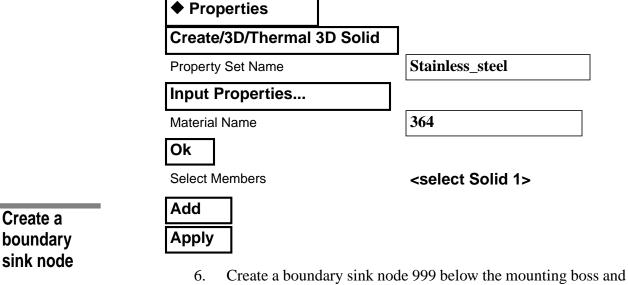
6. Create a boundary sink node 999 below the mounting boss not associated with geometry.
