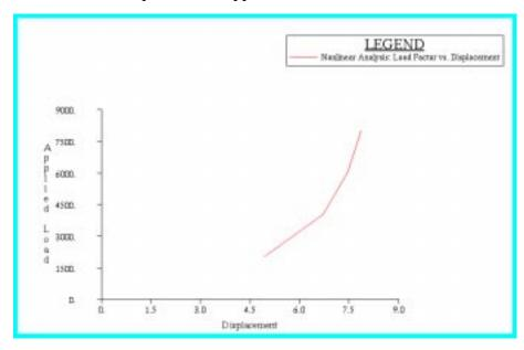
Notice that there is no longer a linear relationship between the displacement and the load factor.
