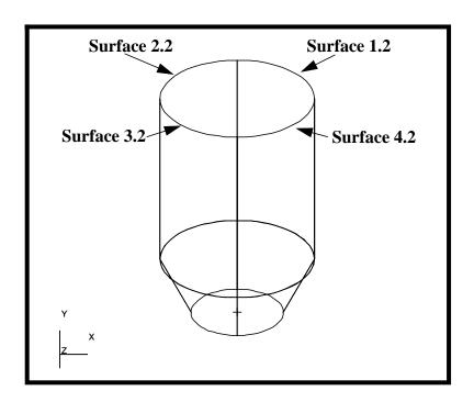
In the vertical direction (y-direction), define a smoothly transitioning mesh density, the elements along the top of the cylinder are 2.5 times as large as those along the bottom edge (tapered end) of the fairing.
