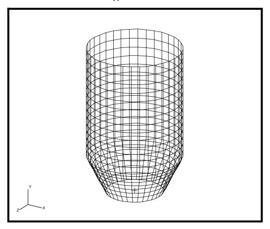
Mesh the horizontal (circumferential) edges of each surface with twonoded bar elements.
