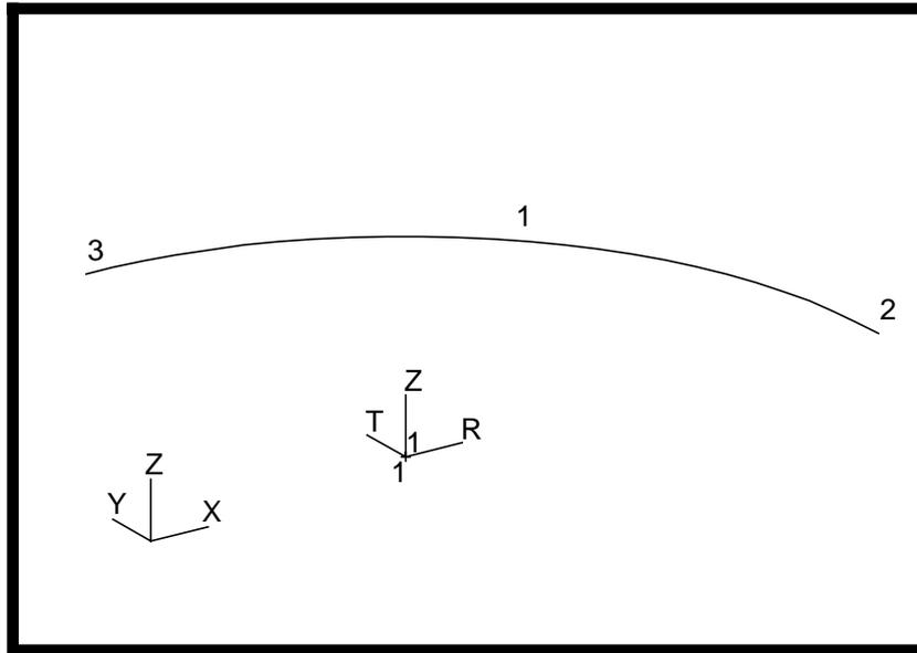
3a. Generate one-quarter of the cylinder wall by extruding the curve created in the previous operation.
