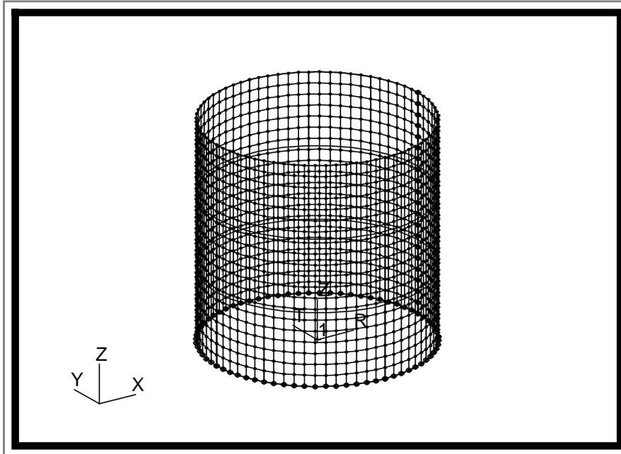
Remember to equivalence the model to remove duplicate nodes at common surface edges.
