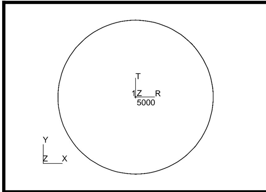
8. Next, create an RBE3 element to distribute the load from the load application node to the cylinder walls.
