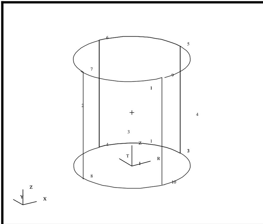
4. Before you mesh the model, plant mesh seeds to define the size of the elements. Note that the mesh seeds will have precedence over the **Global Edge Length** parameter in the *Create/Mesh* form. You may wish to make the nodes that will be generated during the meshing operation more visible. Do this by changing the node size using the **Display/Finite Elements...** option.
