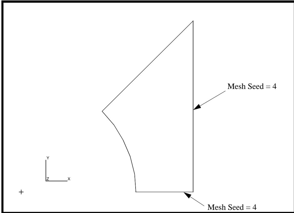
4. Create two mesh seeds on the newly created surface. Use a Mesh Seed of 4 on the vertical and the horizontal edges.
